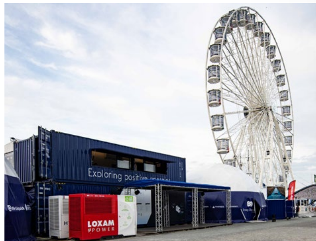
Hydrogen generator powering an exhibition village and the big wheel at the start of the Route du Rhum.
